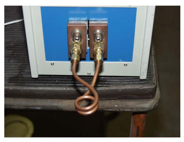
Regular Coil, for brazing router bits, shaper cutters
